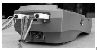
**WARNING:** - There is **ONLY** one correct way to connect the 'K' type thermocouple plug into the socket (see 2.4). The thermocouple plug is designed with one thick (negative) and one thinner (positive) prong. Forcing the plug into the socket the wrong way round may result in damage to the instrument. **Failure to comply may result in damage to the instrument and will invalidate the warranty.**
