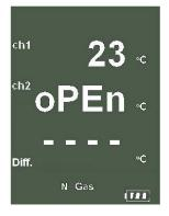
Displays Temperature reading of Channel 1 (ch1) in degrees Centigrade ( $^{\circ}$ C) Displays Temperature reading of Channel 2 (ch2) in degrees Centigrade ( $^{\circ}$ C) Displays the Differential Temperature (Diff.) between ch1 and ch2 in  $^{\circ}$ C
