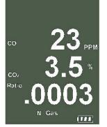
Displays Carbon Monoxide (CO) reading in parts per million (ppm) Displays calculated Carbon Dioxide (CO<sub>2</sub>) figure in percentage (%) Displays calculated CO/CO<sub>2</sub> (Ratio) figure
