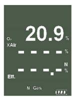
Displays Oxygen (O<sub>2</sub>) reading in percentage (%) Displays calculated Excess Air (X Air) figure in percentage (%) Displays calculated Efficiency (Eff.) figure in percentage (%)
