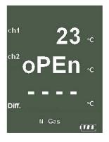
Displays Temperature reading of Channel 1 (ch1) in degrees Centigrade (°C) or degrees Fahrenheit (°F) Displays Temperature reading of Channel 2 (ch2) in degrees Centigrade (°C) or degrees Fahrenheit (°F) Displays the Differential Temperature (Diff.) between ch1 and ch2 in °C or °F
