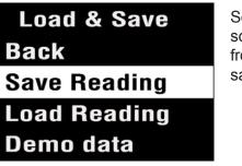
Selecting **Save Reading** opens a screen that allows the user to choose from one of 3 Memories in which to save the reading.
