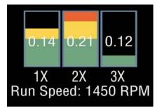
Pressing the square button brings up a display similar to that shown opposite, which shows the readings of vibration velocity (mm/s or inch/s) broken down into each of 3 bands.
