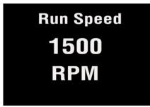
The first screen to be displayed shows the running speed in the previously selected units (Hz or RPM).
