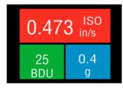
Taking a reading causes the overall vibration numbers screen to be displayed as shown in the example screen left.
