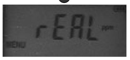
"REAL" mode will display leak levels in ppm (parts per million)
