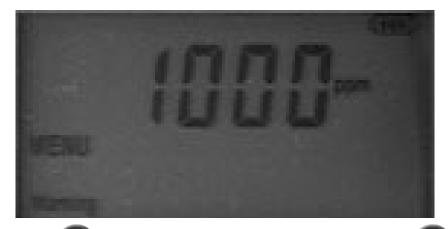
4. Press the MUTE key to increase the alarm level or the ZERO key to decrease the alarm level. The alarm can be adjusted from 100ppm to 5000ppm in increments of 100ppm. Press the key when finished.
