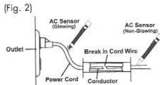
As you move the plastic probe tip away from the electrical source, in this case the wall receptacle, the probe tip will stop glowing at the exact break point in the wire. (Fig. 2)
