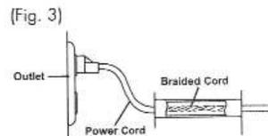
Round electrical cords that contain a twisted conductor internally will cause the AC Sensor to glow, stop glowing, and glow again, as the probe tip is moved along the length of the cord. This is due to the spiral of the conductor wire that produces voltage. (Fig. 3)
