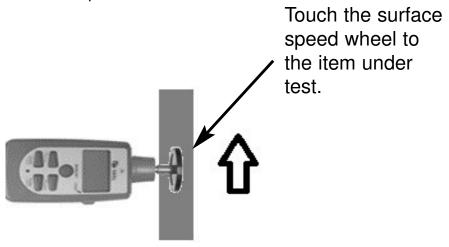
Note: In this mode the meter displays the surface speed in ft/min (feet per minute) or m/min (meters per minute) and not RPM. Do not use the surface speed wheel to measure RPM. Displayed readings will be incorrect.
