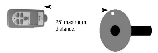
Maximum distance to target is dependent on several items like the strengh of reflection of the laser, ambient light conditions, and the surface of the item under test. For best results the background surface should be dark as compared to the reflective tape. If readings are unstable, move closer to the target for better performance. At long distances a tripod or other rest may be necessary for proper function.
