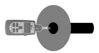
Lightly press the cone or concave tip to the center of the rotating shaft. Measuring from anywhere but the center will result in incorrect readings.
