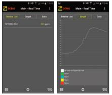
**TPI Smart Probe App** Use the TPI app to display real time readings in numeric and graph format.
