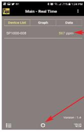
Displays the measured CO2 in ppm.
