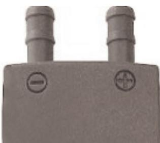
The inputs are marked + and -. Any pressure connected to the - port will be subtracted from the + port. For standard pressure / vacuum measurements use the + port only. Use the + and - port when performing differential measurements.
