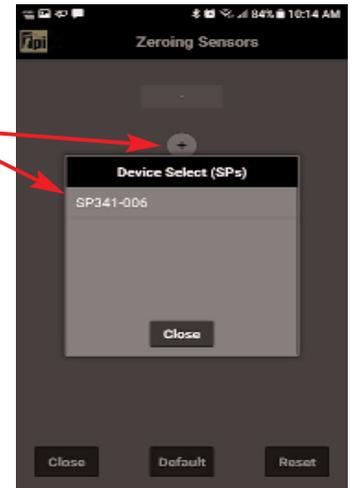
7. Tap the Reset icon to set the pressure reading to 0 (+/- 0.05 counts)
