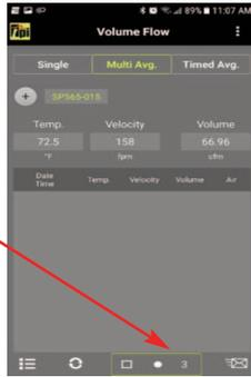
7. Slowly pull the probe towards the entrance point of the duct. Stop at each point and press the “Point” icon to record the reading.
