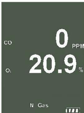
Displays Carbon Monoxide (CO) reading in parts per million (ppm)
