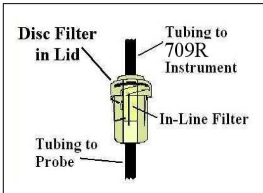
This consists of a Particle Filter in the Bowl Compartment and a Disc Filter in the Lid (as shown in the diagram across). The Disc Filter in Lid will prevent any excessive water from entering the 709R Combustion Analyser if used correctly.
