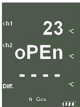
Displays Temperature reading of Channel 1 (ch1) in degrees Centigrade (°C) or degrees Fahrenheit (°F)
