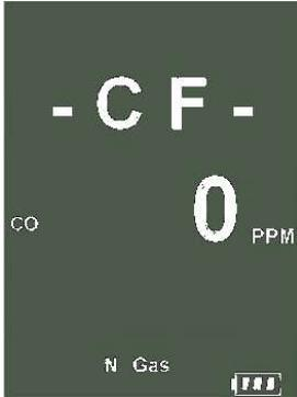
Displays CO air free calculated reading
