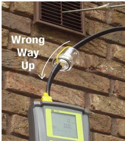
**WARNING:** - There is **ONLY** one correct way to connect the 'K' type thermocouple plug into the socket (see 2.4). The thermocouple plug is designed with one thick (negative) and one thinner (positive) prong. Forcing the plug into the socket the wrong way round may result in damage to the instrument. **Failure to comply may result in damage to the instrument and will invalidate the warranty.**
