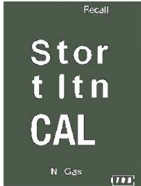
'**Stor**' will be flashing on the display. If you wish to review the Last Time Calibrated Date then press the **Down**
