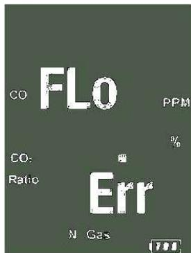
**The 709R will also give off an audible Beeping Alarm to warn that a "FLO Err" is being detected**
