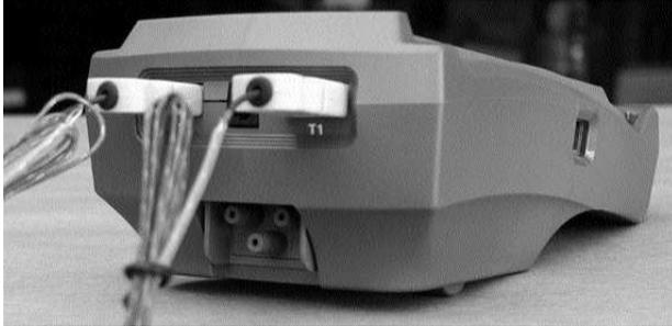
**WARNING:** - There is **ONLY** one correct way to connect the 'K' type thermocouple plug into the socket (see 2.4). The thermocouple plug is designed with one thick (negative) and one thinner (positive) prong. Forcing the plug into the socket the wrong way round may result in damage to the instrument.
