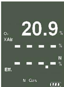
Displays Oxygen (O<sub>2</sub>) reading in percentage (%)
