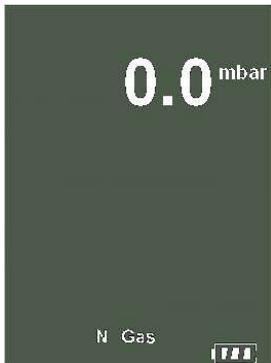
Displays Pressure reading in either millibars (mbar), kiloPascals (kPa), or inches of Water (inH<sub>2</sub>O)
