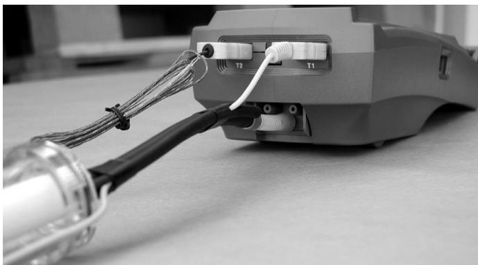
Your temperature-sampling probe comes complete with an In-Line Water Trap Bowl Filter as standard.
