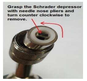
2 Remove and replace the Schrader depressor and/or the worn gasket.
