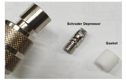
3 Install the gasket and screw in the Schrader depressor. (New Schrader depressor and gasket are part number A670)
