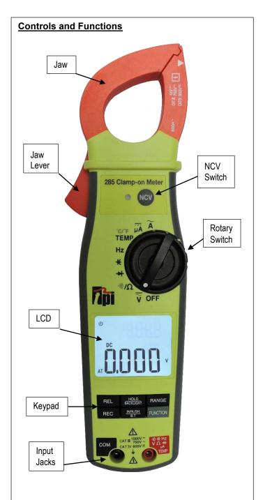
**Jaw** – Used to measure AC Amperage. Place single current carrying wire in the middle of the jaw.
