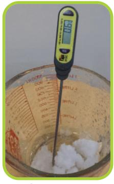
All "C" version digital thermometers can be auto field calibrated in 0° C ice water to ± 1° C
