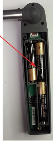
Turn the battery compartment screw counter clockwise until it is just above the compartment door. Lift on the screw to open the compartment.
