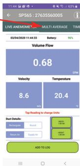
2. Once you've entered the correct Duct Details tap the "Start Test" icon to begin the test process..
