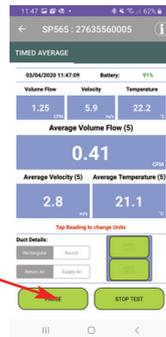
11. When the duct has been completely traversed and prior to pulling the probe out of the last test hole, press the “Stop” icon.
