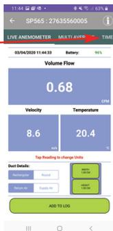
5. Once you've entered the correct Duct Details tap the “Start Test” icon to begin the test process.
