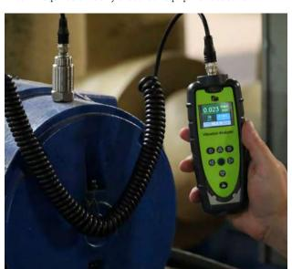
intrinsically safe and complies with BS EN IEC 60079. Hence any CBM equipment needs to be IECEx/ATEX certified for use in hazardous locations.
